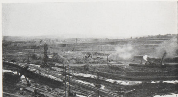
A panoramic view of the vast amphitheatre of the Canadian Johns-Manville mine at Asbestos, which covers an area of 50 acres. It is a shallow mine, and constantly extends as the terraces are cut further back into the rock. Portable railway tracks are laid along the terraces, and dump trains move the broken rock from terrace to mill. When a new terrace is blasted the tracks are moved into the "face". A machine called a "track mover" is gripped to a length of track and in a few minutes it moves the track to the new position, lifting it about two feet at a time, ties and all. In the dim distance, near the centre, is seen a church steeple, a land-mark of the village of Asbestos, which is on the edge of the mine and is gradually being pushed
